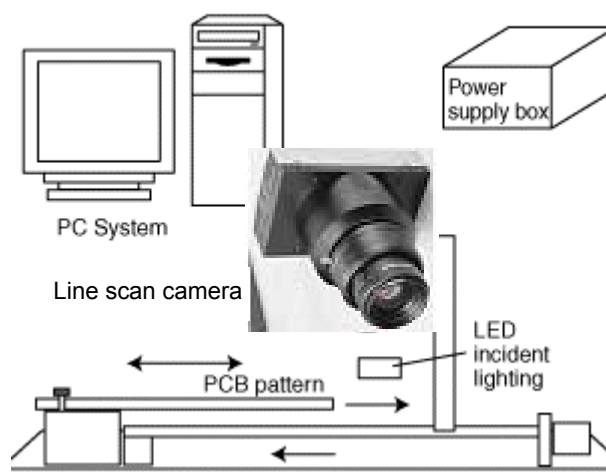
Figure 1-2-1 Visual Inspection of PCBs
